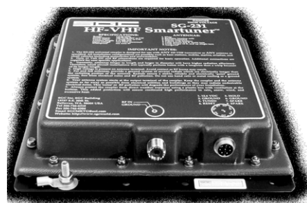
Bottom end, showing the coaxial input socket and the control cable socket.
