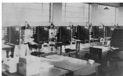
A rare view of the inside of the RSS/SCU (SIS-controlled) Hanslope Park station, with 24 operator positions (22 having two HRO receivers, 2 having three HROs). It became operational in May 1942 and remained so continuously until after VE-day, intercepting mainly the traffic of the Abwehr. This photograph was taken in the summer of 1946, soon after the station was converted for two-way working for what the following year became the Diplomatic Wireless Service. A feature of the station was a set of wideband distribution amplifiers - the first of their type and designed by the late 'Dud' Charman, G6CJ. These amplifiers, using 807 valves as small-signal amplifiers of impressive linearity, remained in use at Hanslope for 30 years without a single 807 ever failing.
