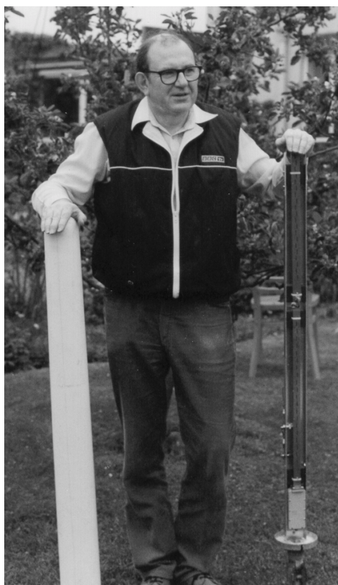
Tom, G3LMX, with the GB3TG 10GHz slot aerials.
